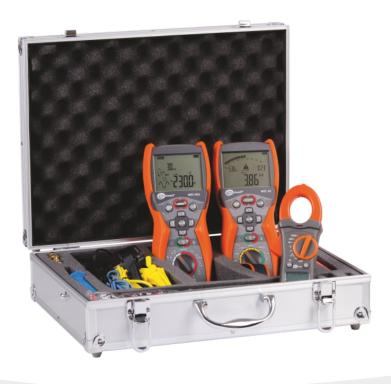
This set allows for performance of measurements in accordance with the HD 60364-6:2008 and EN 61557 standards:
