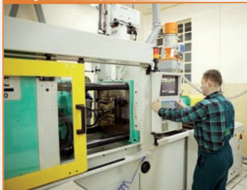
Arburg - mould for plastic parts
